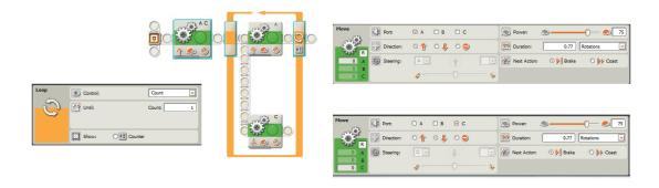
You don't have to put the A & C motors inside a loop, but it makes the turns stand out visually while working in a lengthy program.
