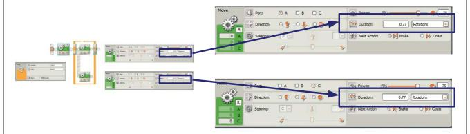
Value of turn in rotations (or degrees) calculated based on the required change in robot heading for each turn of the polygon.
