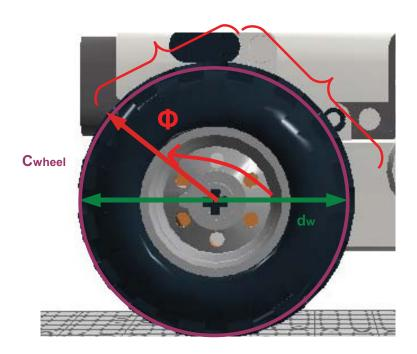
Telling the robot to turn the motor by  $\Phi$  forces the wheel to travel along **C**turn.
